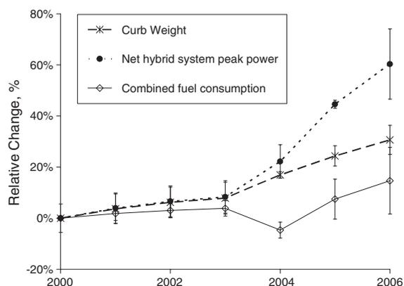
**Figure 2.** Vehicle performance trends over time for the average HEV: curb weight, net hybrid system peak power, and fuel consumption. Variability across models is indicated by the error bars representing one (sales-weighted) standard deviation.
