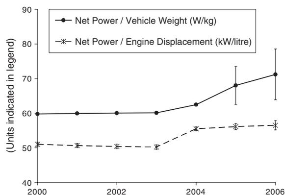
**Figure 3.** Trends in net system power per vehicle weight (a measure of vehicle performance) and net system power per engine volumetric displacement (a measure of the technological development of the propulsion system). Data dispersion is indicated by the weighted standard deviation.
